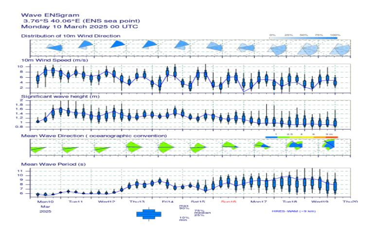
The distribution of wind directions is South East, throughout the 10 days forecast period, the wind speeds vary between 3 m/s and 9 m/s, the wave heights vary between 1.0 m and 1.8 m. The wave directions are Southeasterly (SE) and the wave periods between 5 and 9 seconds
